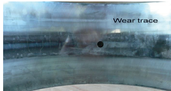
Abrasive wear on outer ring raceway (SRB).
