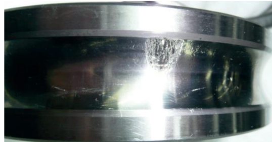
Pitting (Flaking) on the surface of the inner ring raceway. Specific after wrong mounting procedure
