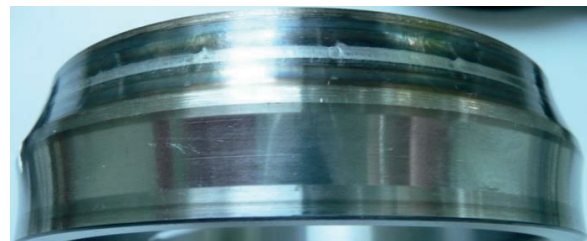
Uneven running pattern of inner ring raceway.
