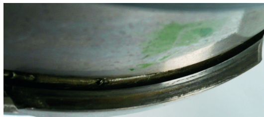
Damaged central flange due to improper mounting (blow)
