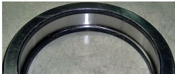
Corrosion while storage.
