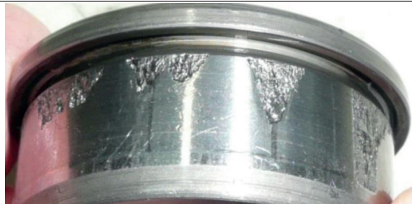
Flaking equally spaced at the rollers pitch on the inner ring. Specific to vibration occurrence during running.
