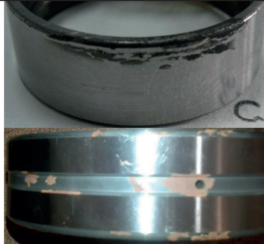
Front and outer corrosion on the outer ring
