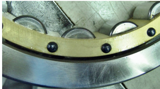
Wear on rollers end face of Cylindrical Roller Bearing.
