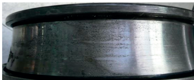
Apparition of pitting (flaking) on the raceway of the inner ring..
