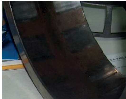
Corrosion while stationary.
