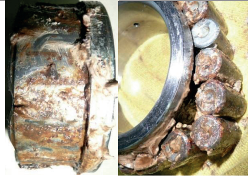
Corrosion. Contaminated lubricant.
