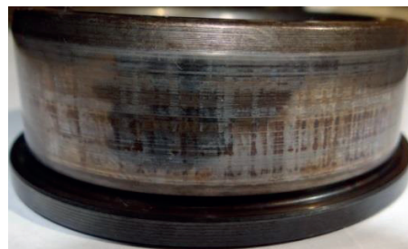
Abrasive wear and vibrations on raceway of a cylindrical inner ring.
