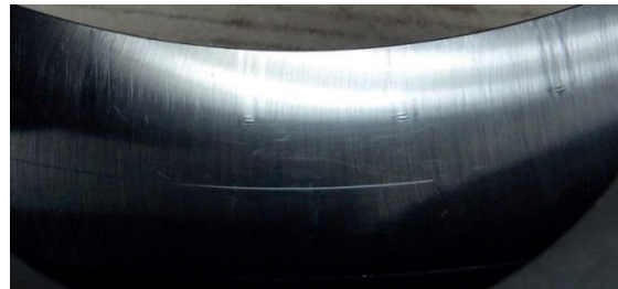
Raceway true brinelling – Spherical roller bearing
