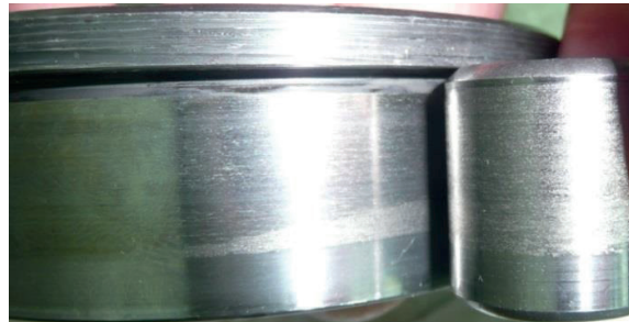
Smearing on inner ring raceway and roller
