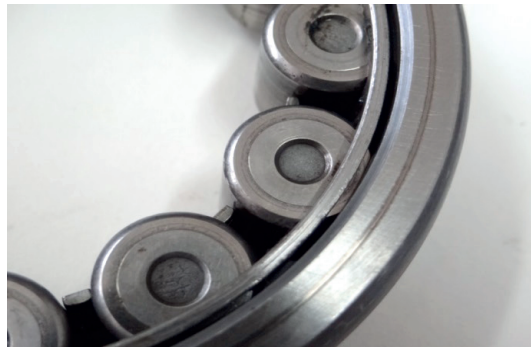
Wear on inner ring rib face and roller and face of Cylindrical Roller Bearing with rib.
